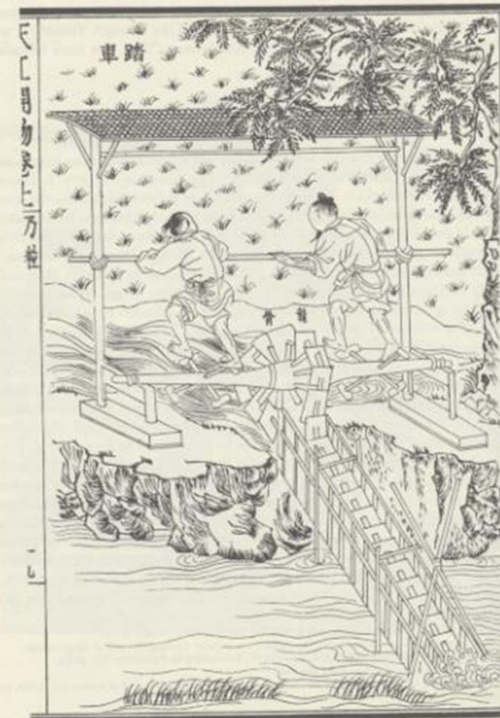
Fig. 579. The square-pallet chain-pump in the Thien Kung Khai Wu of 1637 (ch. 1, p. 190), here called the shui-chi .
